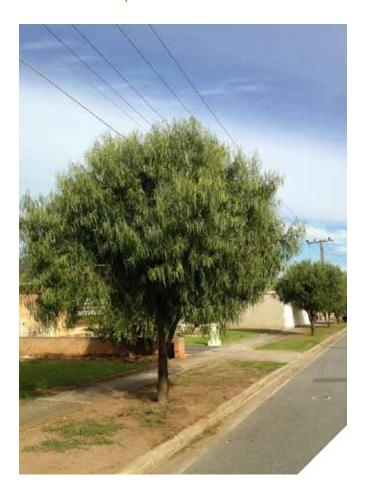
There is a legislative requirement for SA Power Networks to inspect and manage trees under powerlines to minimise risk to life and property and maintain safe power supply. Appropriate management of trees involves ensuring specific clearance zones between the tree crown and the lines. Greater clearances are required in bushfire risk areas and under high voltage lines.
