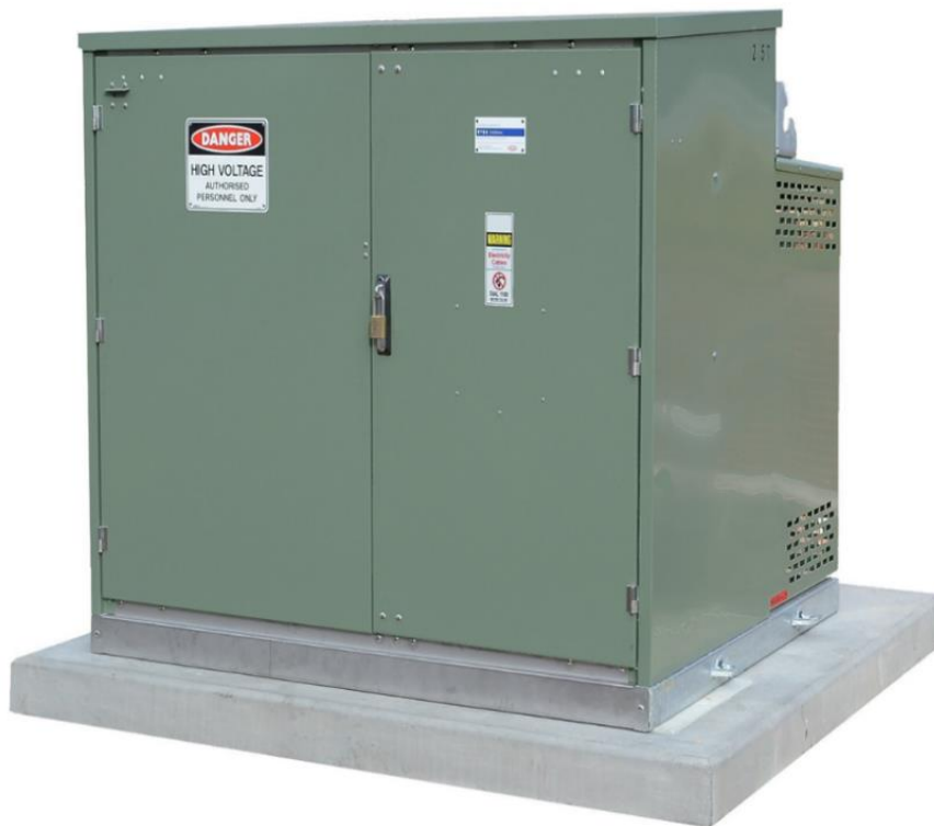
Figure 1 Typical Mk7 Transformer with 'Wilson Ring Main Unit' Transformer Rating: 315kVA to 2000kVA Voltage Ratio: 11kV/0.4kV, 11kV and 7.6kV/0.4kV
