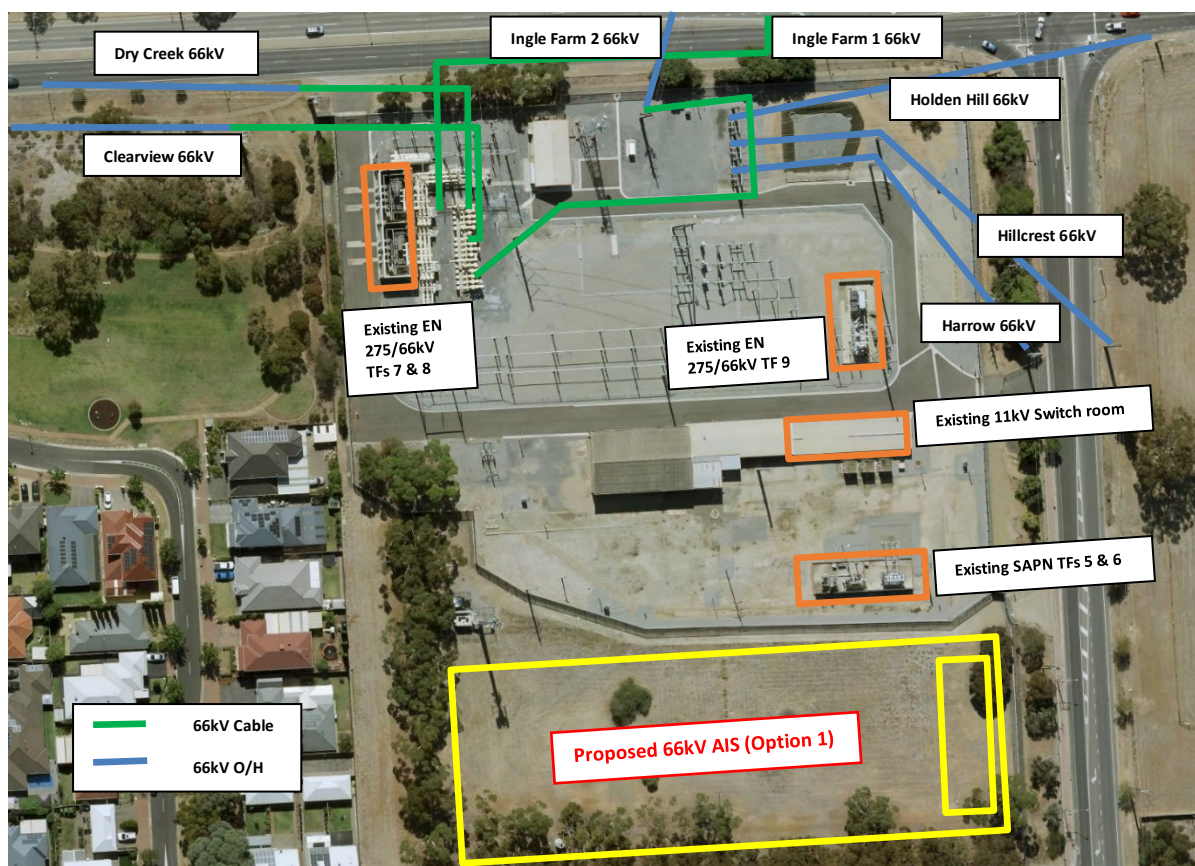
Figure 2.9: Layout of Northfield AIS under Option 1
